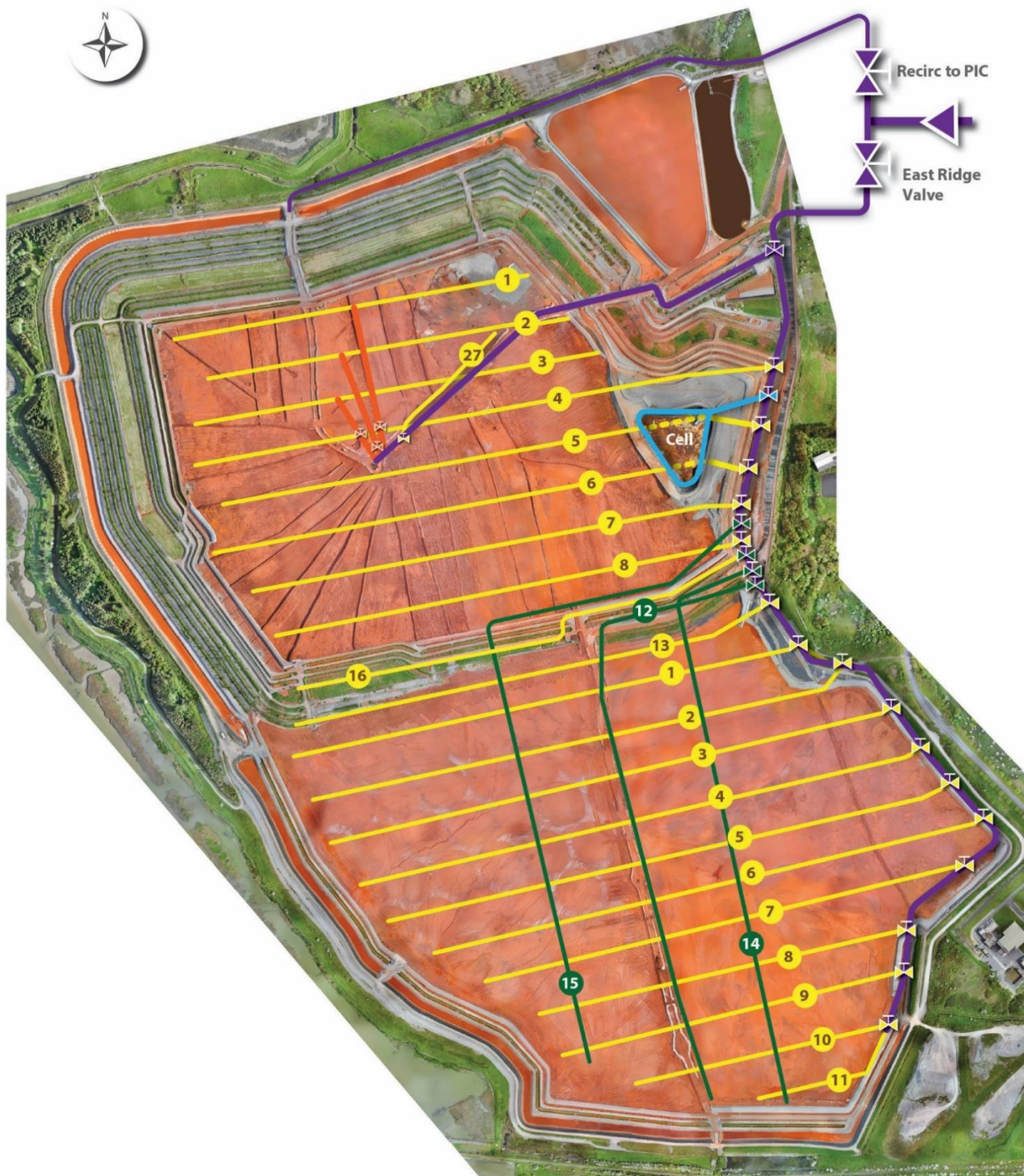
Figure 37: BRDA Sprinkler Line Layout (December 2020)
