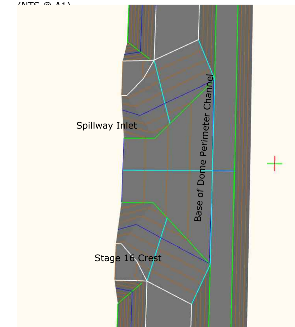
Simplified Spillway Confluence - Liner Formation 3D Model (NTS @ A1)
