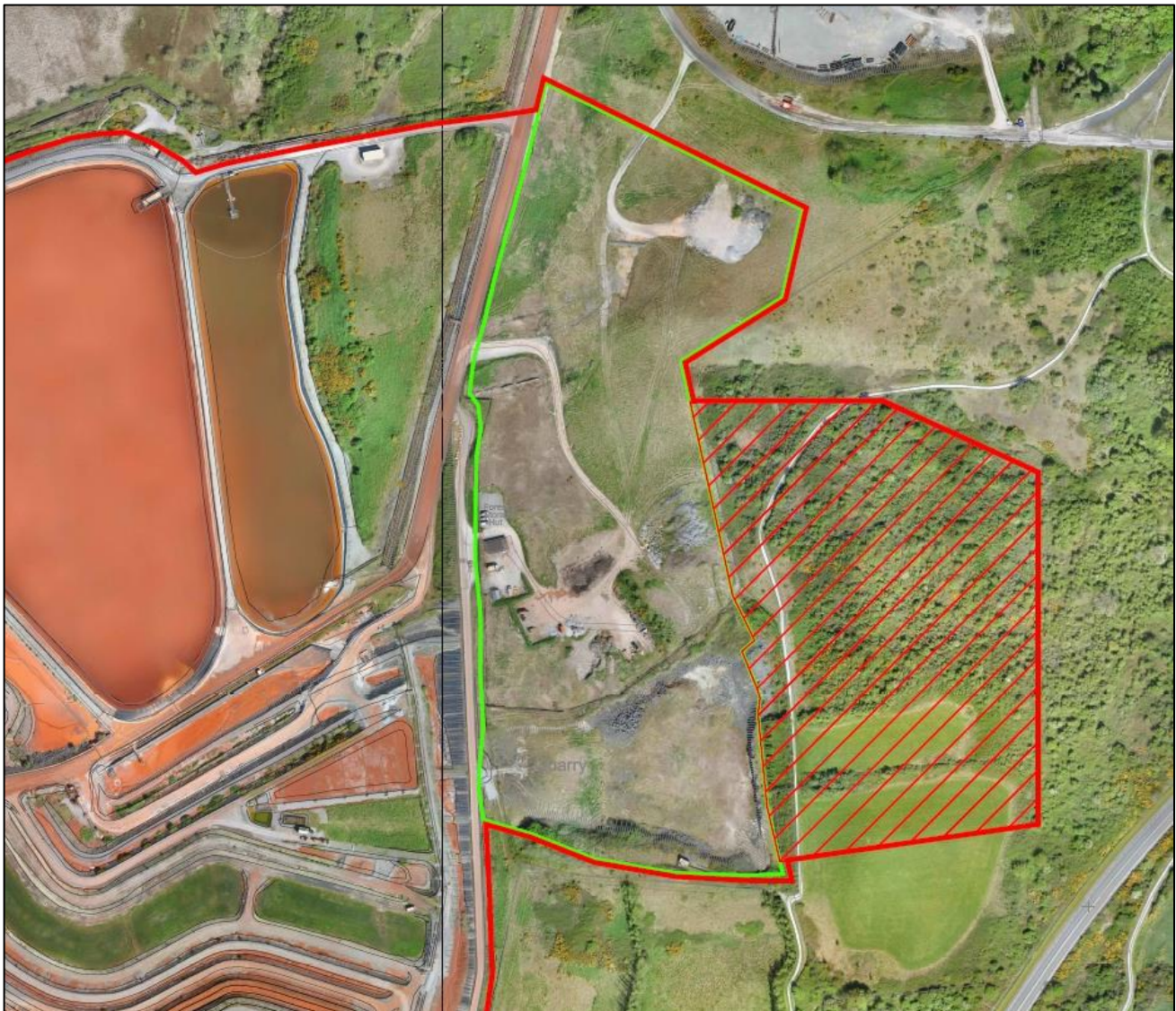
Figure 40: Permitted Borrow Pit Footprint (green) and the Proposed Borrow Pit Extension Footprint (red hatch), April 2021
