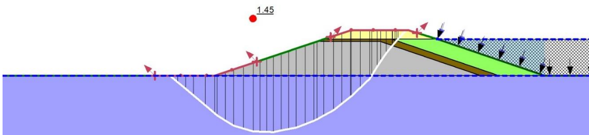
Figure D18: Undrained (Total Stress) Static Analysis (Post seismic) – PIC Failure
